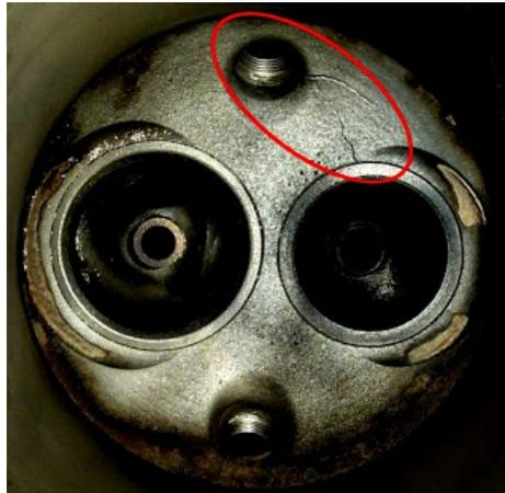
I explained that any non-ferrous metal component (like an aluminum alloy cylinder head) will eventually crack if subject to repetitive stress for a sufficient period of time. The component will crack sooner if the repetitive stress is more intense and/or if the operating temperature is greater. Extended full-power operation during glider tows obviously increases the intensity of the stress, and the very high CHTs reduce the tensile strength of the cylinder head.
