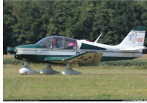
When towing gliders, the airplane climbs at full power and very slow airspeeds, and CHTs regularly register in the high 400s Fahrenheit, close to Lycoming's 500F CHT red line. Once the glider releases, the engine is throttled back to idle and descends rapidly to land and hook up for the next tow.
