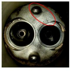
(The head's tensile strength is reduced to 50% of its room-temperature value at a CHT of 400F, and to about 33% at 500F.)
