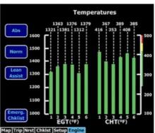
and serious engine damage. If you observe low EGTs and high CHTs after an aircraft comes out of maintenance, do not fly until you've had the ignition timing re-checked.
