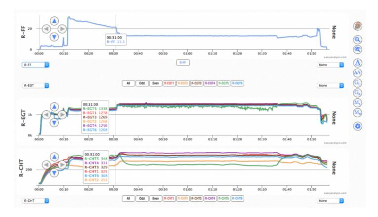
CHT 2 – the gold trace – is using a spark plug gasket probe, so we expect to see lower CHTs. Aside from that all looks ok except EGT and CHT 5. They're high when FF is high, then at the big pull (at the cursor) CHT 5 drops dramatically and EGT 5 becomes jittery.
