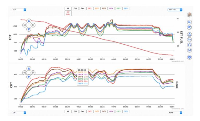
The pilot reported that when he topped off, the panel-mounted fuel gauges read accurately, and as he flew, those gauges showed that he was using more fuel than the engine monitor showed. For instance, he'd top off, reset the EI, fly for an hour with FF around 12-14 GPH, his gauges showed about half-tanks, but the EI showed him down about 12-14 GPH. The longer he flew, the closer to E his gauges would read. If he landed and topped-off, the pump showed 12-14 GPH and the gauges read F again.
