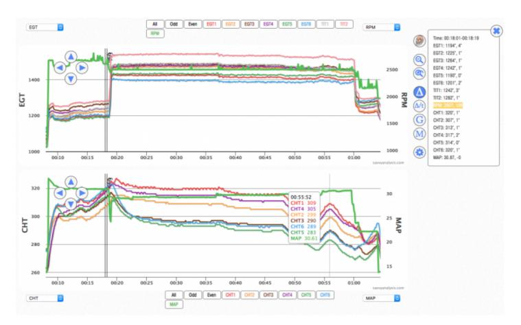
This isn't the entire flight – I zoomed in to show takeoff to approach. The data shows momentary spikes in RPM. The pilot saw the spikes in real time, but felt no surges or change in power when he saw them.
